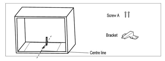
3. Remove the bottom cabinet template and fix the bracket using A screws.
