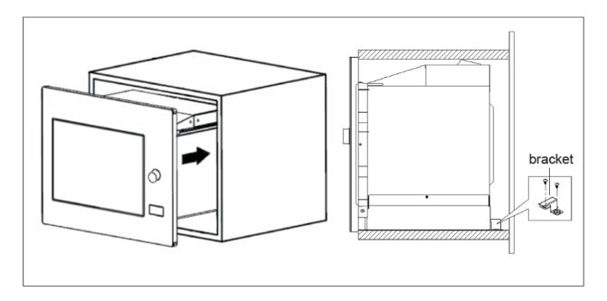
5. Open the door and fix the microwave-oven in the cabinet using B screw, where the installation hole is.
